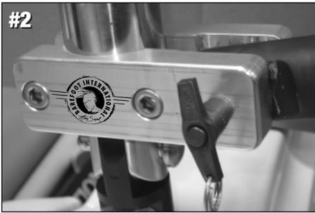
8. Attach both boom arm brace clamps to boom Section A approximately 1 to 3 feet from the boat on the inside boom Section A (See **Photo #1** & **#3**).
